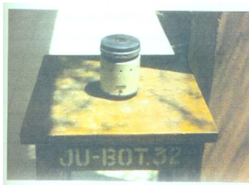
Fig. 1. “Burkard portable spore trap sampler”
