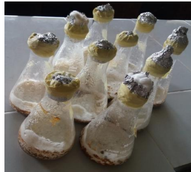
Fig. 2. Laccase production via solid state fermentation using rice bran as carbon source
