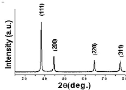
Fig. 4. XRD patterns of silver nanoparticles by treating *C. roseus* var. *alba* callus extract with  $\text{AgNO}_3$  aqueous solutions
