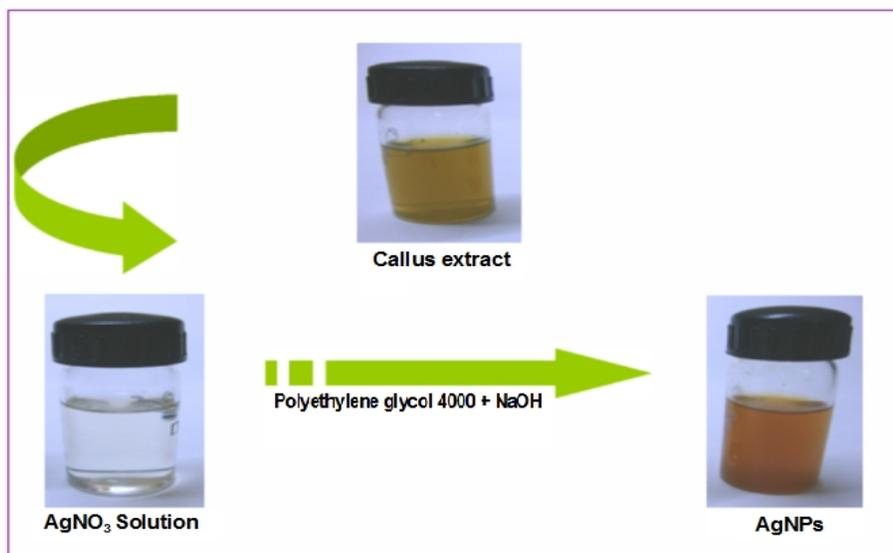
Fig. 1. Green synthesis of silver nanoparticles
