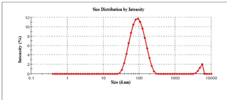
Fig. 3. Particle size distribution of Silver Nanoparticles synthesized by *C. roseus* var. *alba* callus extract
