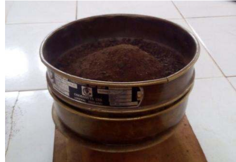
Plate 1. The assemblage of the sieving process
