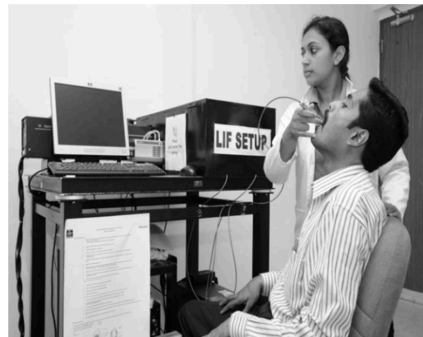
Fig. 2 Block diagram and the Photograph of the He-Cd laser based tabletop LIF system.
